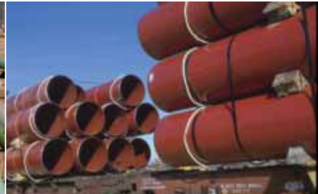
Large diameter pipe with fusion bond epoxy coating in Western Canada
