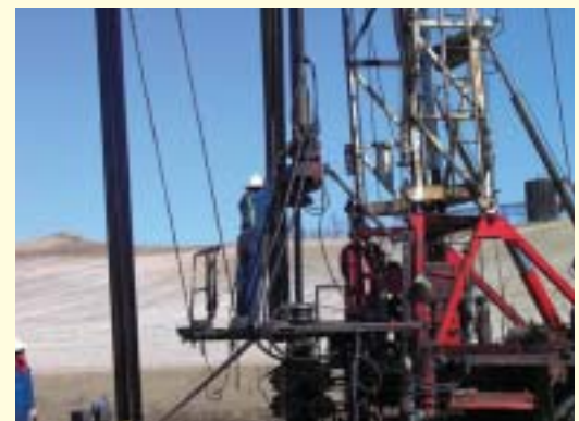
A Guardian technician utilizes an over-the-well inspection unit to check production tubing as it is removed from the well.
