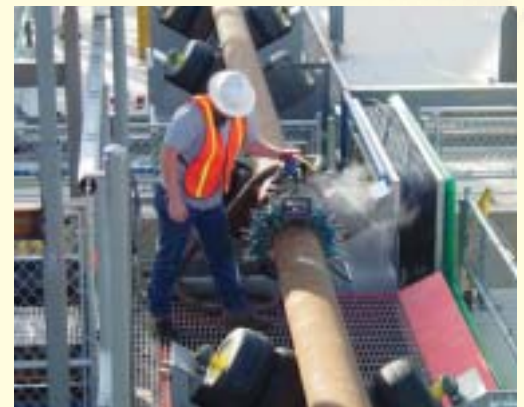
A technician monitors the ultrasonic transducer array utilized to inspect a pipeline girth weld.
