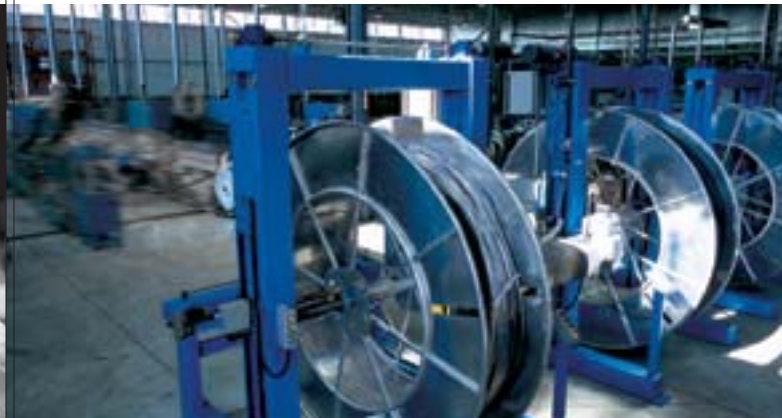
HIGH CAPACITY TAKE-UP REELS ARE UTILIZED TO ALLOW LONGER PRODUCTION RUNS OF CONTINUOUSLY EXPANDED, HEAT SHRINKABLE TUBING.
