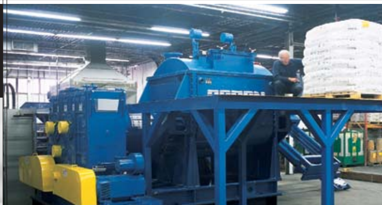
NEW, HIGH CAPACITY ADHESIVE MIXER PROVIDES INCREASED CAPACITY TO MANUFACTURE PIPELINE SLEEVES AT THE CANUSA - CPS FACILITY IN HUNTSVILLE, ONTARIO.
