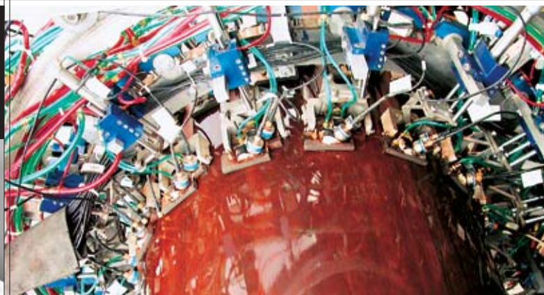
COMPLEX TRANSDUCER ARRAY UTILIZED TO TRANSMIT AND RECEIVE ULTRASONIC SIGNALS THROUGH THE PIPELINE GIRTH WELD.
