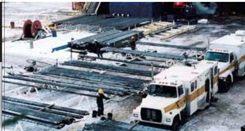
GUARDIAN TECHNICIANS UTILIZE PORTABLE, COMPUTERIZED DRILL PIPE INSPECTION EQUIPMENT UNDER DEMANDING CONDITIONS AT REMOTE RIG SITES.
