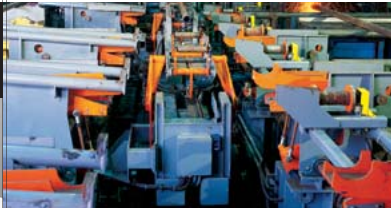
OMSCO'S NEW, ROBOTIC PIPE HANDLING SYSTEM FEEDS SEAMLESS STEEL TUBES INTO THE DIVISION'S NEWEST UPSETTER.
